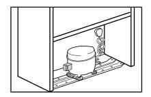
the compressor. (See diagram) Gently remove the plug from the receptacle. Never pull the mains cord, you may damage the appliance. In the case of transportation, ensure you locate the plug in the receptacle provided to avoid transit damage.
