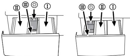
**i** The detergent dispenser may be in two different types according to the model of your machine as seen above.
