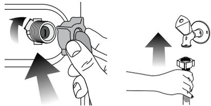
3. Open the taps completely after making the hose connection to check for water leaks at the connection points. If any leaks occur, turn off the tap and remove the nut. Retighten the nut carefully after checking the seal. To prevent water leakages and damages caused by them, keep the taps closed when the machine is not in use.
