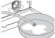
• Pull out the pump outlet hose from its housing.
