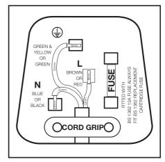
**5.** With alternative plugs a 13 A fuse must be fitted either in the plug or adaptor or in the main fuse box. If in doubt contact a qualified electrician.
