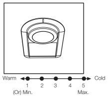
0=System cooling is off. 1=Lowest cooling setting (Warmest setting). 5=Highest cooling setting (Coldest setting).
