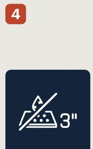
Reset the full filter indicator by pressing it for 3 seconds.
